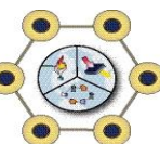
ChaoJi Vehicle Connector Layout Source: White Paper of ChaoJi EV Charging Technology - State Grid Corporation of China and China Electricity Council
