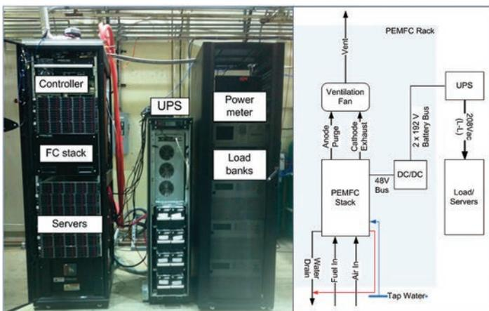
In-Rack Test Unit and System Schematic
