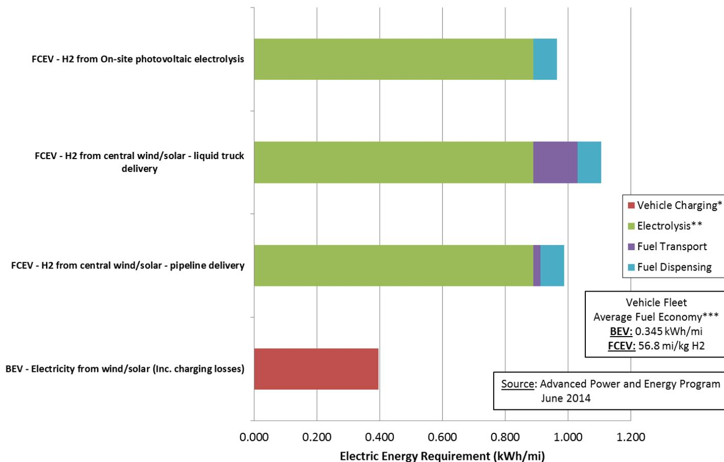
\* Includes energy required to overcome losses in electric vehicle charging equipment in addition to the vehicle energy requirement.
